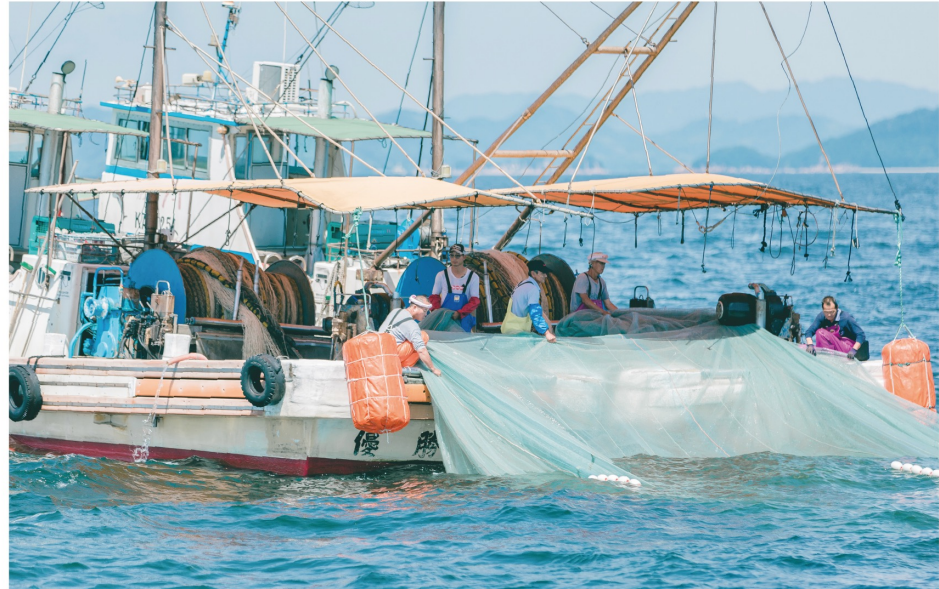
Fishing with a floating trawl net which connects two fishing boats and landing the fish with a net hauler and human power.
